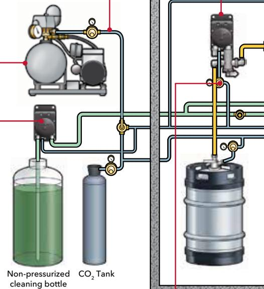
**Pump can also be utilized to aid** in beer line cleaning through wall mounted cleaning sockets.
