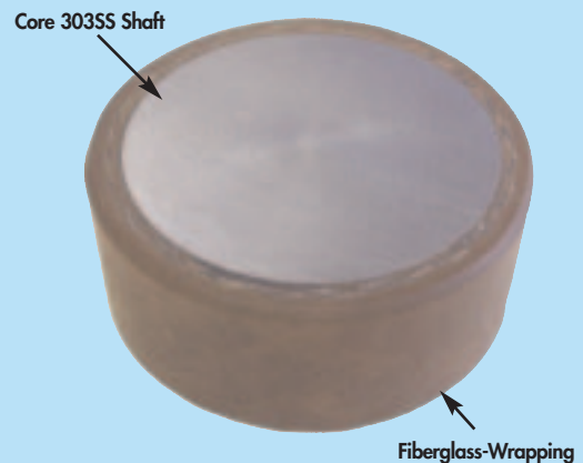
Figure 3 - Cross-section of a fiberglass-wrapped 303SS shaft. The cross-section shows the core, non-wetted, 303SS shaft and is meant to highlight the shaft's substantial fiberglass-reinforced wrapping, greater than 1/8" (3.2 mm).
