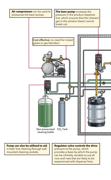
Flojet's BeerJet pumps are capable of pumping beer up to 240 meters horizontal or 30 meters vertical through a single line. The pump can dispense up to five taps from a single keg and has a service life of more than 250,000 liters.
