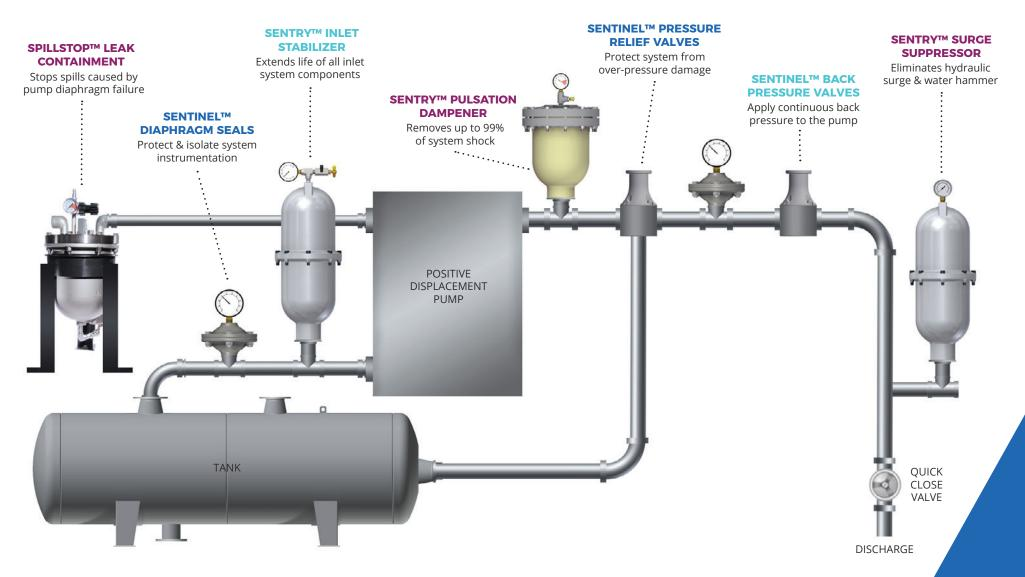
Installation of the pulsation dampener should be no more than ten pipe diameters from the pump's discharge. Additional pump system diagragm featuring the Hybrid Valve™ configuration is available on page 29 of this guide.
