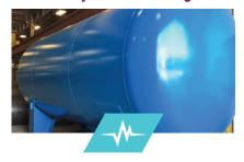
Compressor style surge vessels contain detection instrumentation and allow for additional or less air into the tank to adjust for a change in the fluid level.
